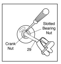
driver in one of the slots in the slotted bearing nut. Lightly tap the screwdriver with a hammer to turn the slotted bearing nut counterclockwise until the arms are no longer loose. **Do not overtighten the slotted bearing nut.** When the slotted bearing nut is properly tightened, tighten the Crank Nut.
